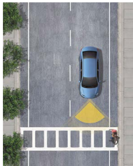
PRE-COLLISION SYSTEM 23 WITH PEDESTRIAN DETECTION 24 (PCS w/PD)
